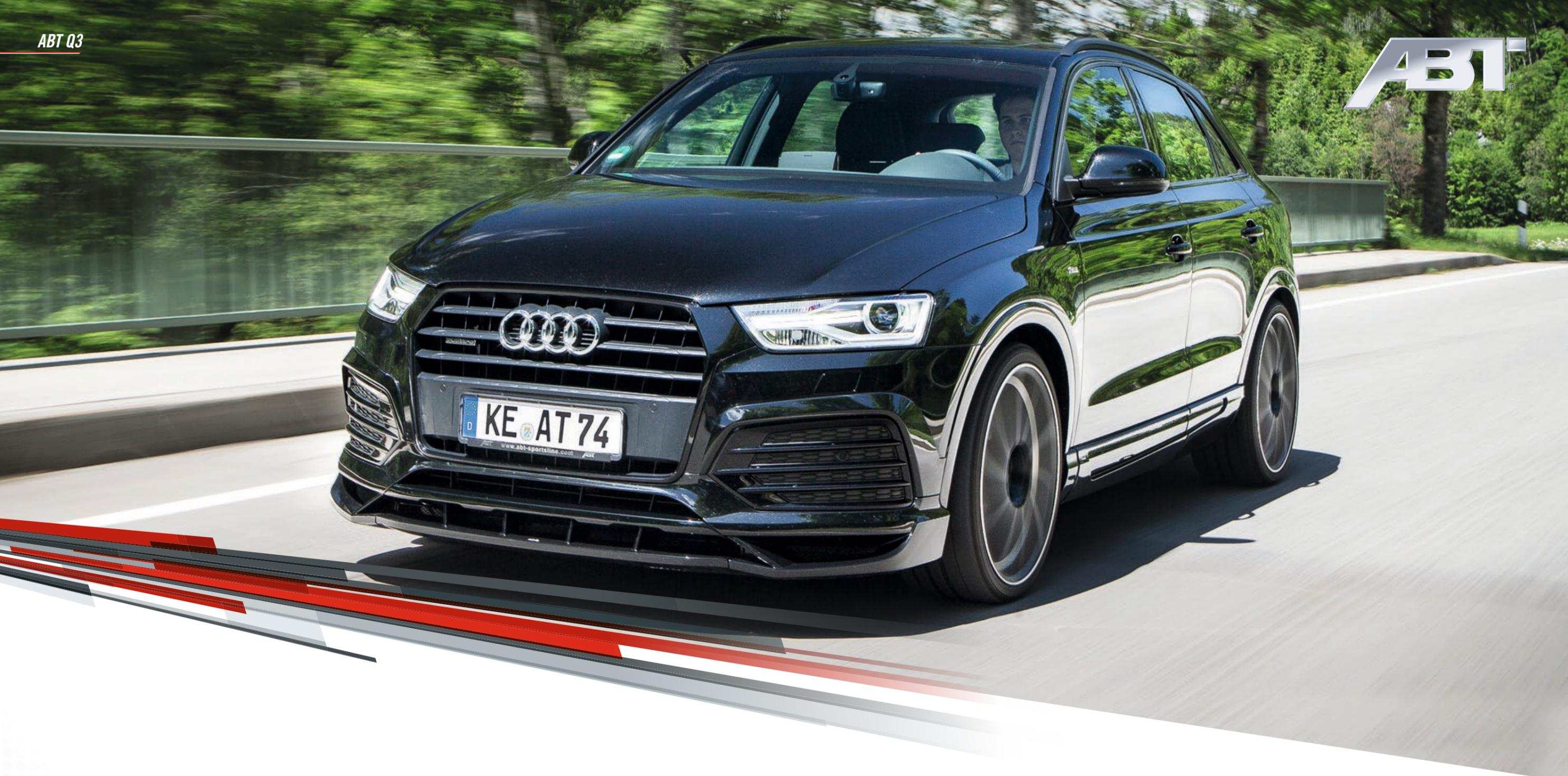
The springs, lowering the Q3's CoG by about an inch, have a huge effect on its handling, for example. The car now corners as if it is on rails. If you want even more raciness, use the ABT height adjustable suspension kit. Depending on how you drive, the car's CoG can be lowered by one to two inches on the front axle and 1 ½ to 2 ½ inches on the rear.
